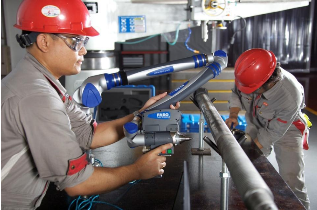
Picture 15: Bay 1 –Faro Arm – Component Scanning
