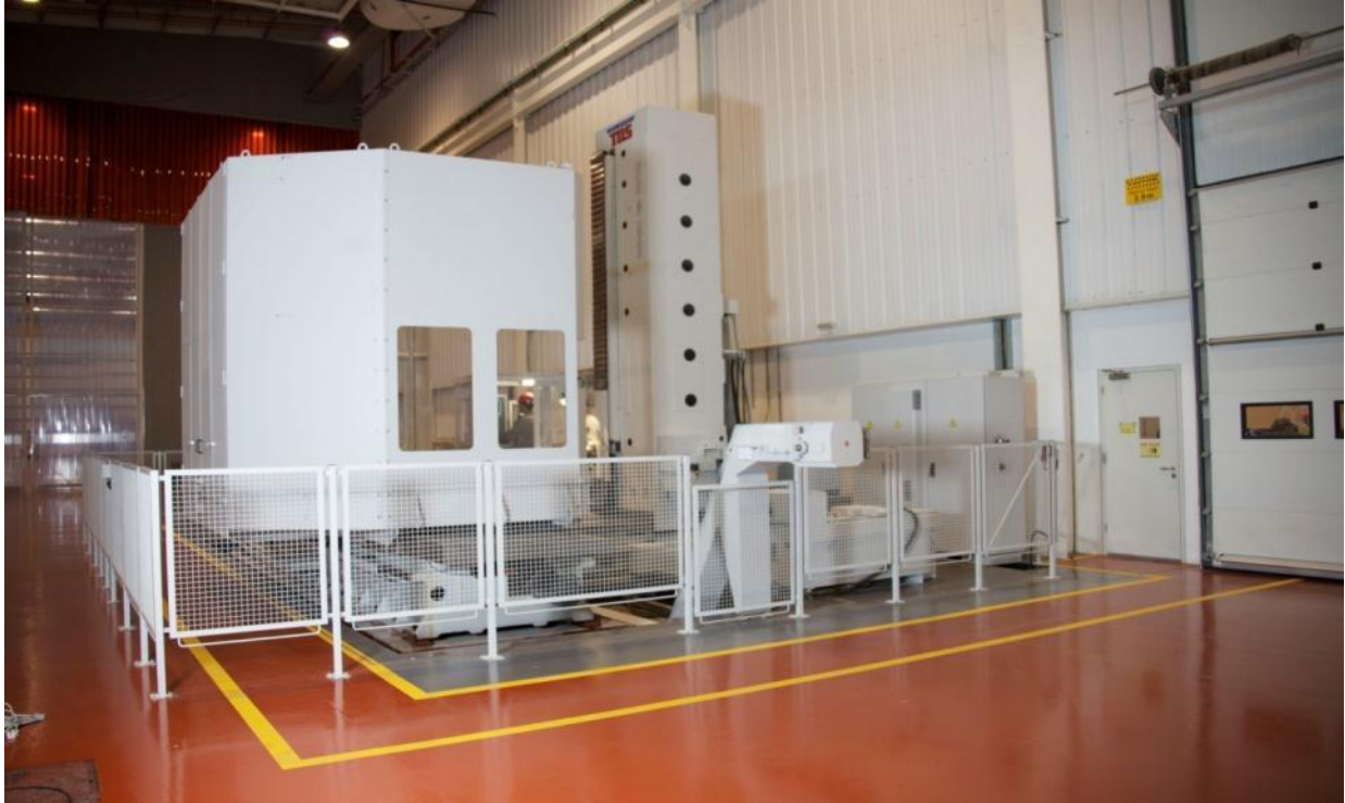
Picture 13: Bay 1 - TOS Varnsdorf WHN 13.8 CNC Horizontal Table Borer and Milling
