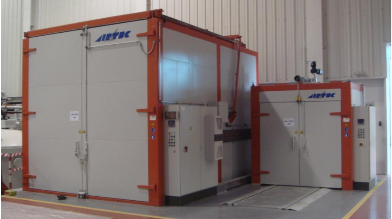
Picture 19: Bay 4 - Curing Ovens - Large and Small
