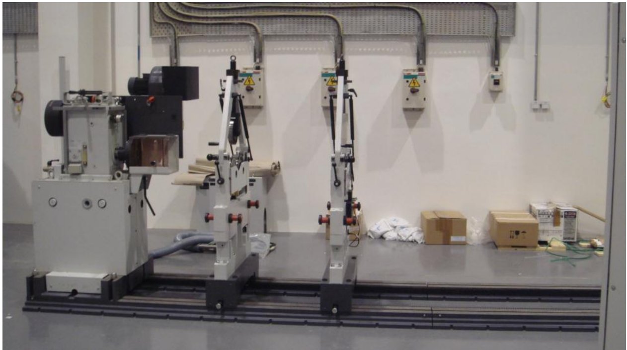
Picture 20: Bay 4 -Schenck HM 60 U/BU Balancing Machine for Low Speed balancing of Rigid Rotors up to 20,000KG
