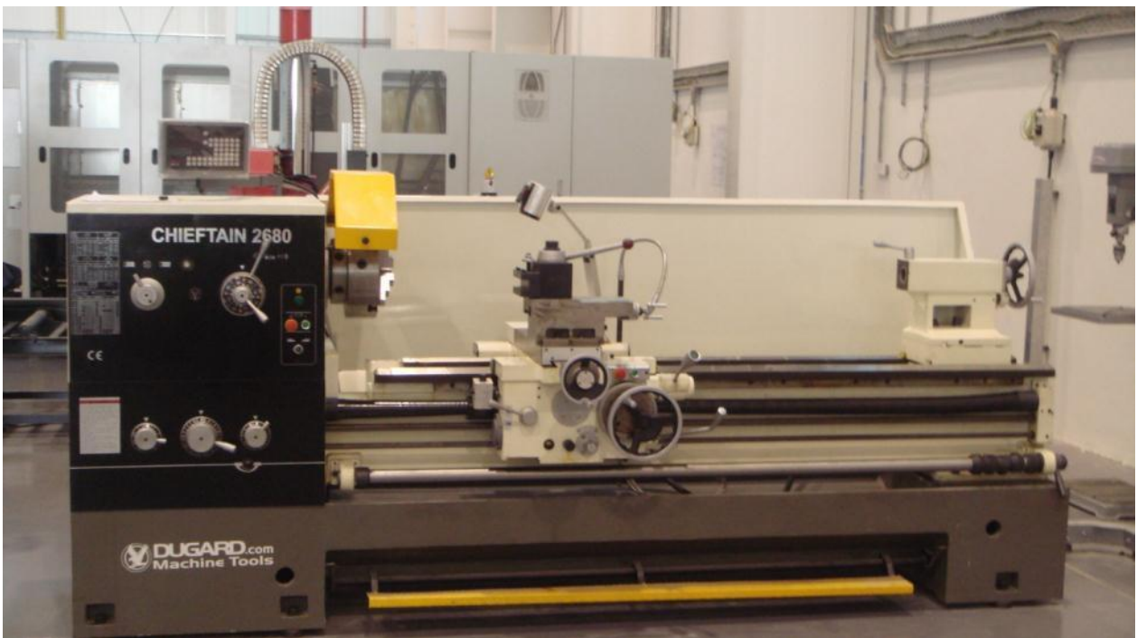
Picture 12: Manual Chieftain Lathe Valiant 2620 with DRO
