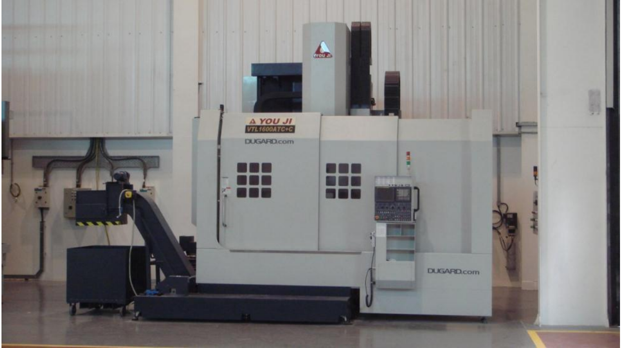
Picture 7: Bay 1- CNC Vertical Machine Centre VTL 1600ATC+C
